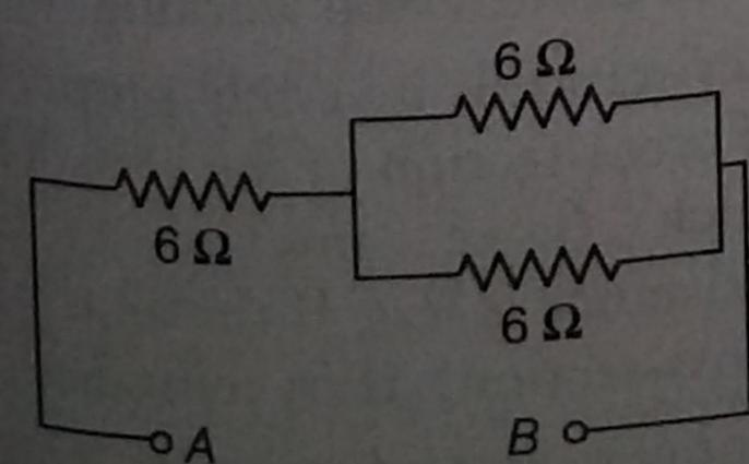
This combination is connected in series with a  $6\Omega$  resistor to get overall equivalent resistance of  $(6+3)=9\Omega$ .
