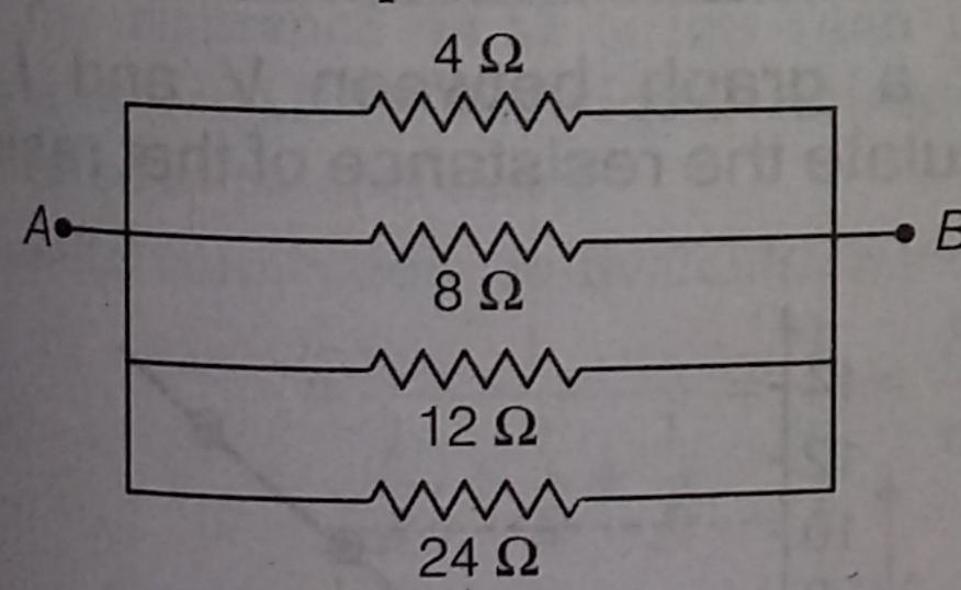
$$R_{\min} = 1/\left[\frac{1}{4} + \frac{1}{8} + \frac{1}{12} + \frac{1}{24}\right] = \frac{24}{12} \Omega = 2\Omega$$
