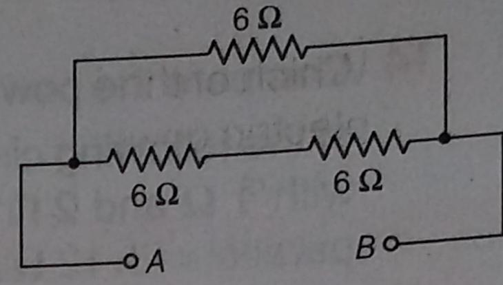
$R' = 6 + 6 = 12 \Omega$ . Now, 12  $\Omega$  and 6  $\Omega$  resistors are connected in
