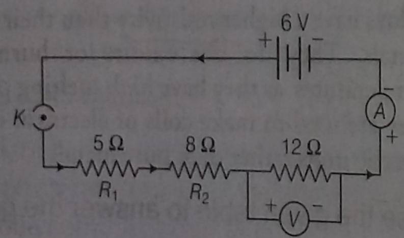
Equivalent resistance of the circuit,
